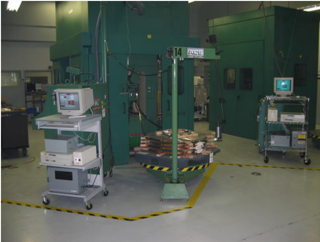
Figure 1. Two SmartPress manufacturing automation systems in use. Each system includes a PC with DAQ board, electrical isolation hardware, battery backup and a barcode printer.
